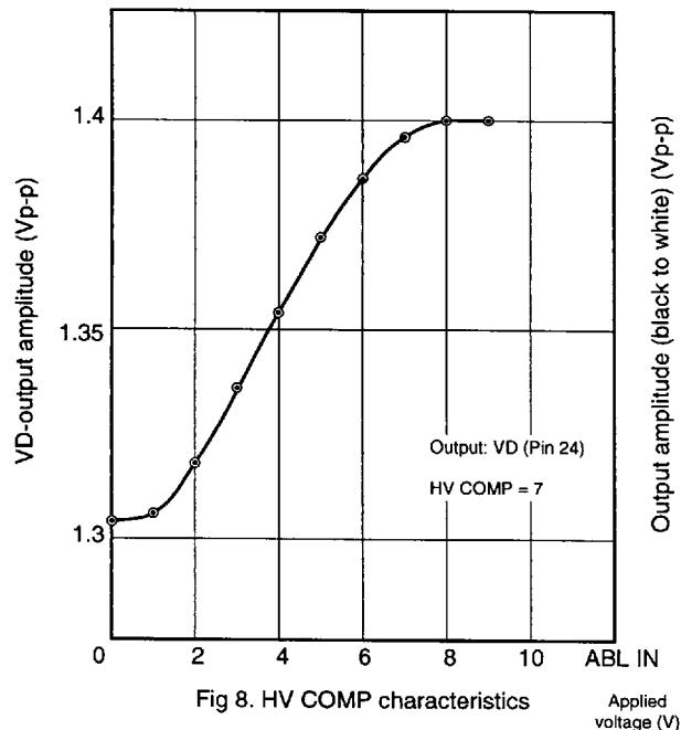
Fig 8. HV COMP characteristics
