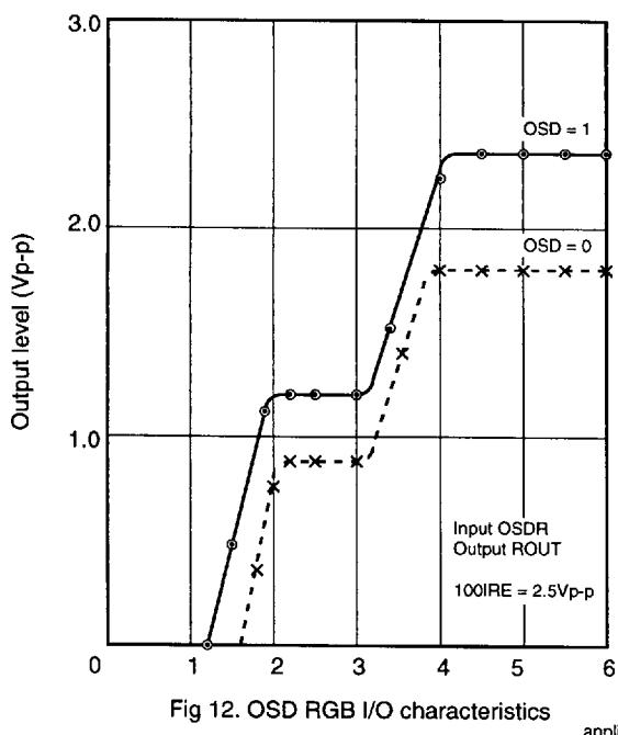
Fig 12. OSD RGB I/O characteristics
